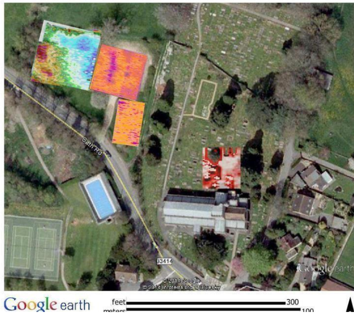
Figure 3.25. Overhead view, showing resistance survey in churchyard, and resistance and radar surveys in church car park. The features here are lower and well separated from the church.
