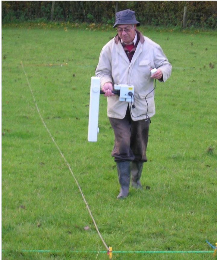
Fig 2.1 Geoscan FM256 magnetometer being operated by John Oswin
