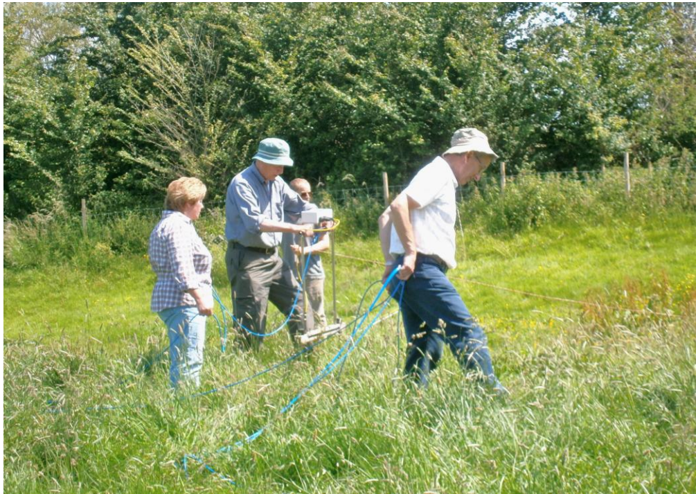
Fig2.2 TR/CIA twin – probe resistance meter being operated by members of the U3A
